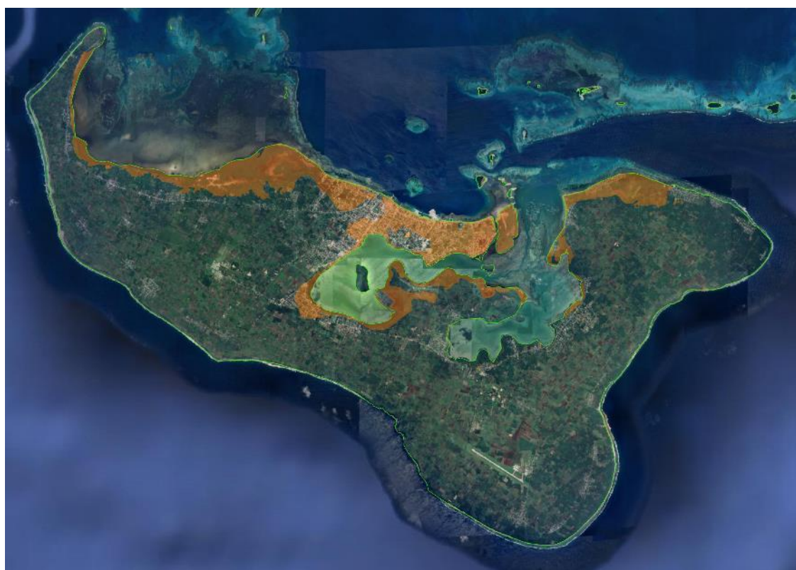
Figure 22 Inundation modelling in Tongatapu under RCP8.5 / 2100
