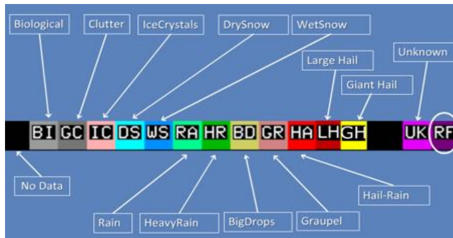
Figure 11. Hydro-meteor classification. (Source: US NWS)
