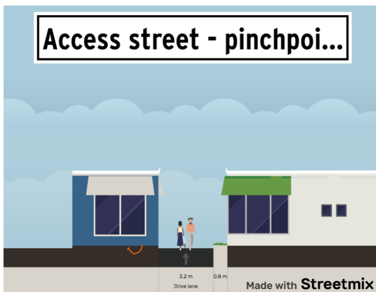
Figure 8-5: Indicative cross section for a pinchpoint on an access street.
