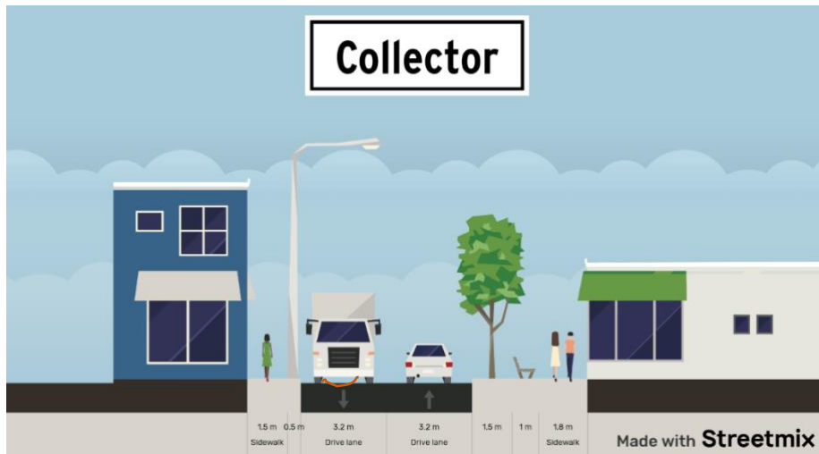
Figure 8-2: Indicative cross section for a collector road.
