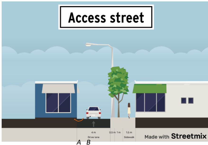
Figure 8-4: Indicative cross section for an access street.
