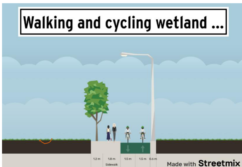
Figure 8-7: Indicative cross section for a walking and cycling pathway above the wetland.
