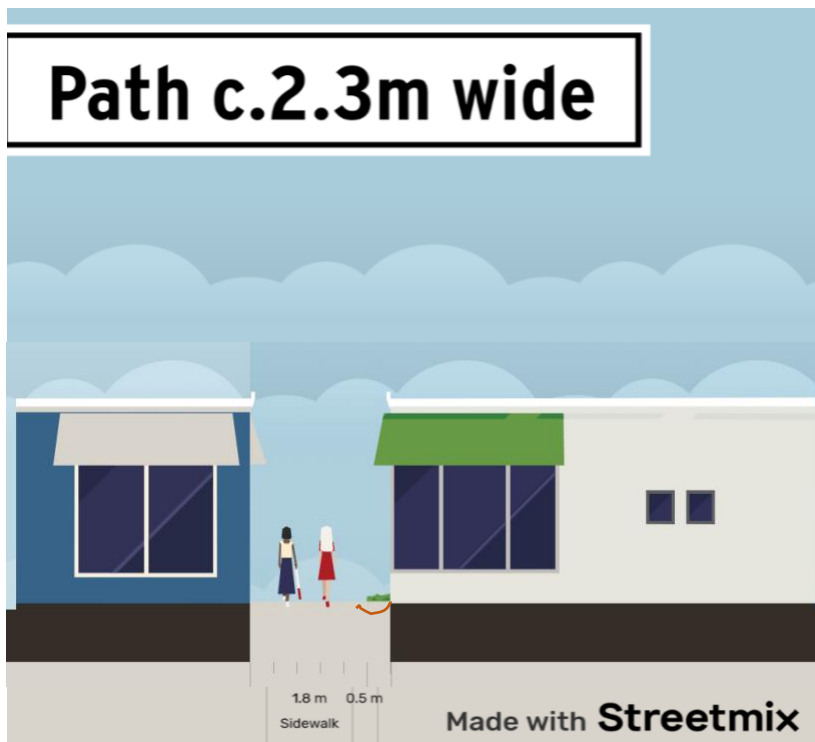
Figure 8-8: Indicative cross section for a path.
